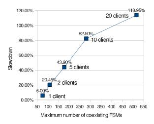
Figure 5: Fixing trace size to 500MB, varying the number of dbench clients
