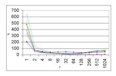
Figure 2: Allan deviation for 8 AMD processors
