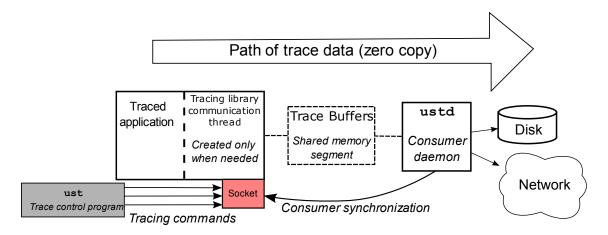
Figure 1: Overview of the LTTng Userspace Tracer architecture.
